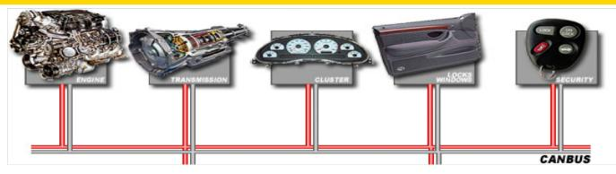
The Controller area network (CAN-bus) is provided with:
