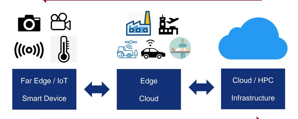
Federating far edge resources ad hoc via wireless (5G, mesh) to provide cloud resources close to the edge
